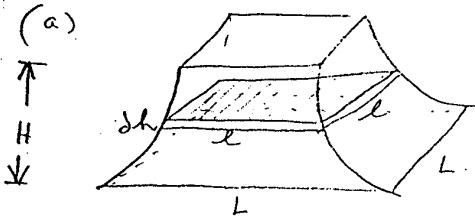
Consider a horizontal slice of side length  $l(h)$  and thickness  $dh$  taken parallel to the base
